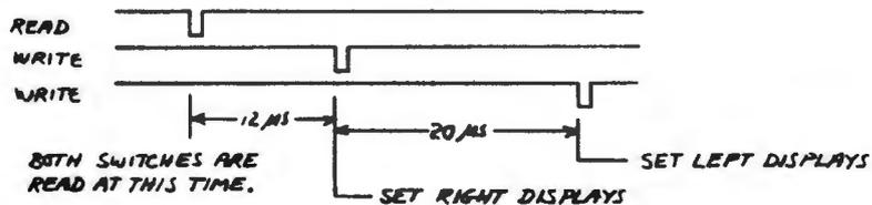
NOTE: TWO ADJACENT DISPLAYS ARE SET BY EACH WRITE STROBE. THE DATA TO THE LEFT ONE IS CLEARED, SO IT SHOULD SHOW "0" DURING THIS TEST.
