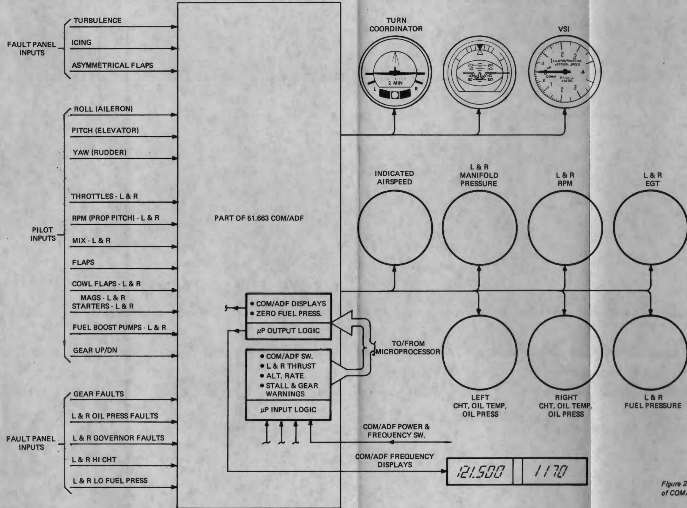
Figure 2.3 Block Diagram of COM/ADF Major Functions
