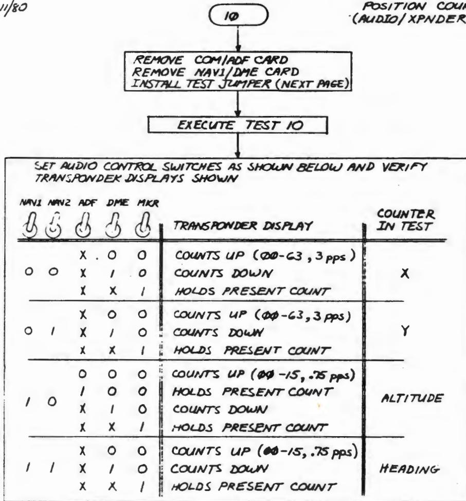
NAV1 & NAV2 SWITCHES ARE READ BY THE TEST PROGRAM TO DETERMINE WHICH COUNTER TO DISPLAY.
