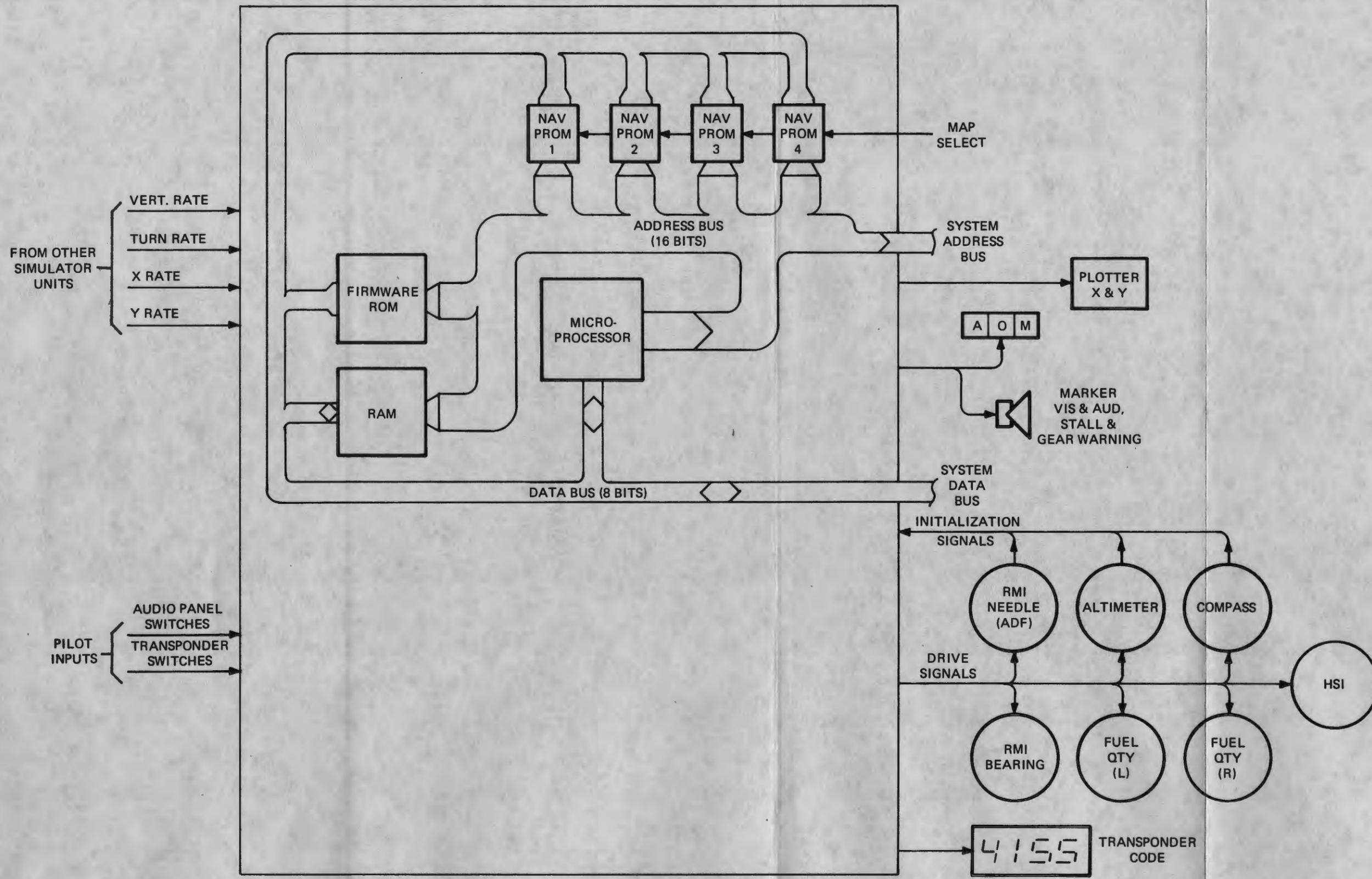
Figure 2.2 Block Diagram of Audio/XPonder Major Functions
