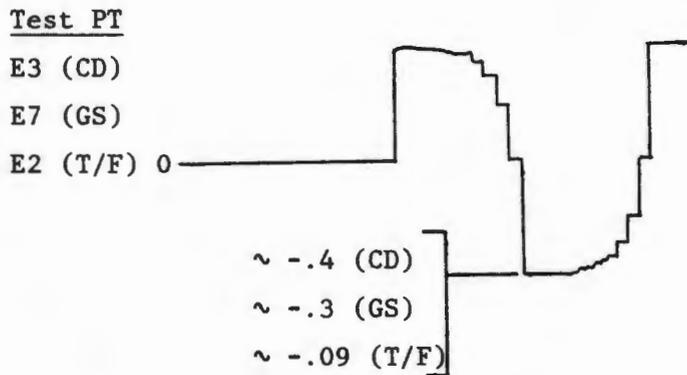
DAC waveforms with meter unplugged.
