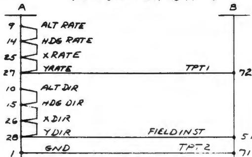
A & B ARE CONNECTOR BLOCKS, .125 X .25 SPACING, CUT DOWN FROM 542.1836
