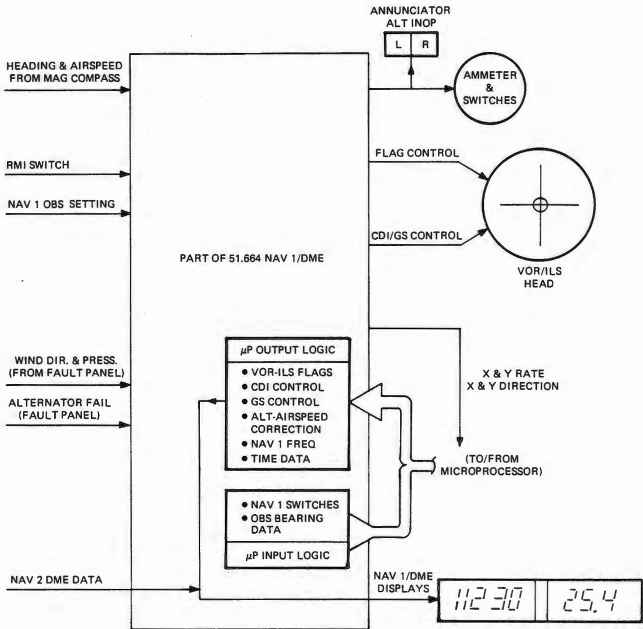
Figure 2.4 Block Diagram of NAV 1/DME Major Functions
