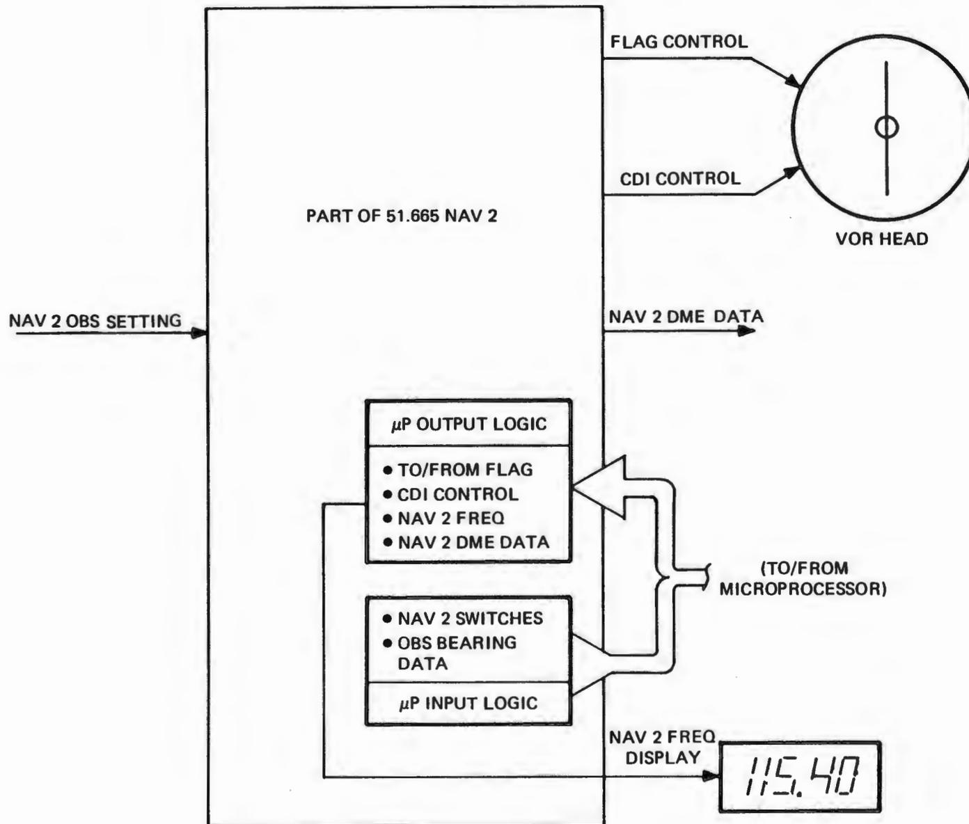
Figure 2.5 Block Diagram of NAV 2
